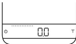
In the Weighing Mode, the scale will only display weight, in either grams or ounces.
