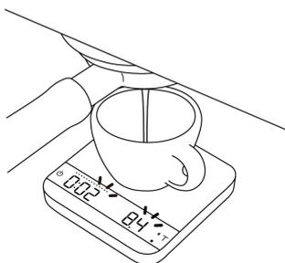
**3** The timer starts when the flow of espresso is detected.
