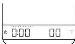
In the Dual Display Mode, the scale displays [ 0:00 0.0 ] with a timer (left) and weight (right).
