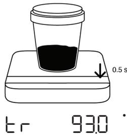
2 Press and hold Tare button for 0.5 second. The scale will display the weight to be deducted.
