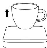
When brewing is completed and the cup is removed from the scale, the display will flash to show the final beverage weight and the average flow-rate of the brewing. The Flow-Rate Indicator will show the average flow-rate with a stripe LED and the highest peak flow-rate with a single bright LED.
