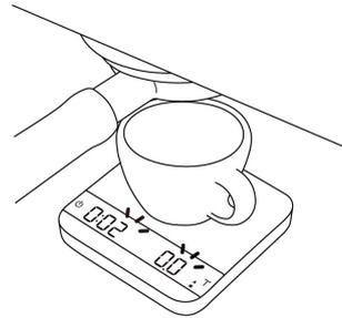
**2** Place a cup on the scale. The scale will perform auto-tare and start the timer.
