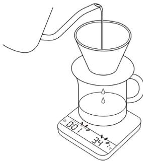
**3** The timer will start automatically when the first flow of water is detected.
