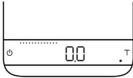
In this mode, the scale will only perform auto-tare. Put the cup on the scale and auto-tare will be performed. Pull the shot of espresso as you normally would. When the cup is removed from the scale, the espresso brewing summary will be displayed.
