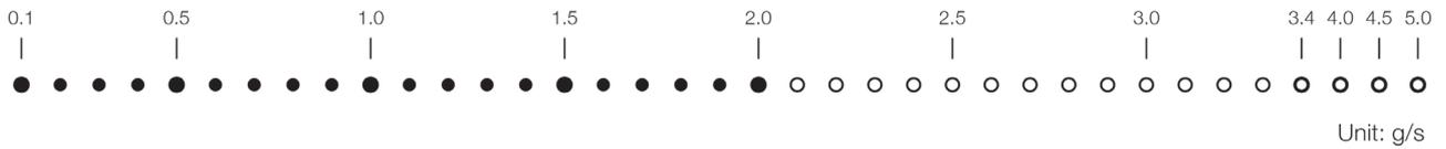
The Flow-Rate Indicator is an LED bar on the top of the display. It helps you visualize your espresso flow-rate in real time and spot channeling during brewing.
