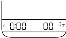
This mode is designed to aid pour over coffee brewing. The scale detects the start of the flow from kettle into vessel and automatically starts the timer. The timer stops when the brewing equipment is removed from the scale. After removing the equipment, the display flashes the final beverage weight.
