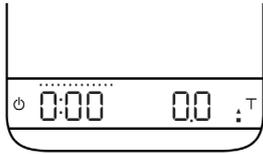
This mode is for baristas to measure the total time of a shot including the pre-infusion time. After a cup is placed on the scale and the weight reading is stable, the scale performs auto-tare and starts the timer.
