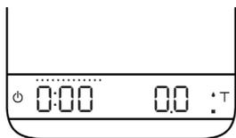
This mode is designed for baristas who would like to measure the time of the shot starting from the first few drops of espresso. When the weight reading is stable, the scale will perform the auto-tare operation. After the scale detects the espresso flow, the timer starts automatically. The timer will stop automatically when the espresso flow stops.
