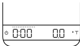
When the scale detects the flow of espresso, the timer starts. The timer will stop when the flow stops.
