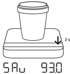
2 Press and hold Tare button for 2 seconds when reading is stable. The weight is stored as a preset container weight.
