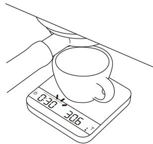
**4** The timer will stop automatically when the espresso flow stops or the cup is removed.
