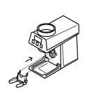
To adjust the portafilter fork, loosen the knobs and change the position until it holds the portafilter in place. Tighten the knobs to lock it into
