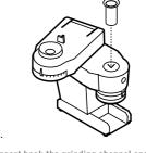
Insert back the grinding channel and its lid by following the guides.
