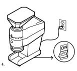
activating the main power switch (placed under the base).
