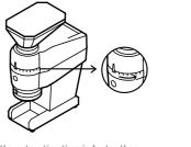
25-30 sec you are likely to have a too coarse grind and need to adjust it to make it finer. Adjust the grind by rotating the top wheel counterclockwise.
