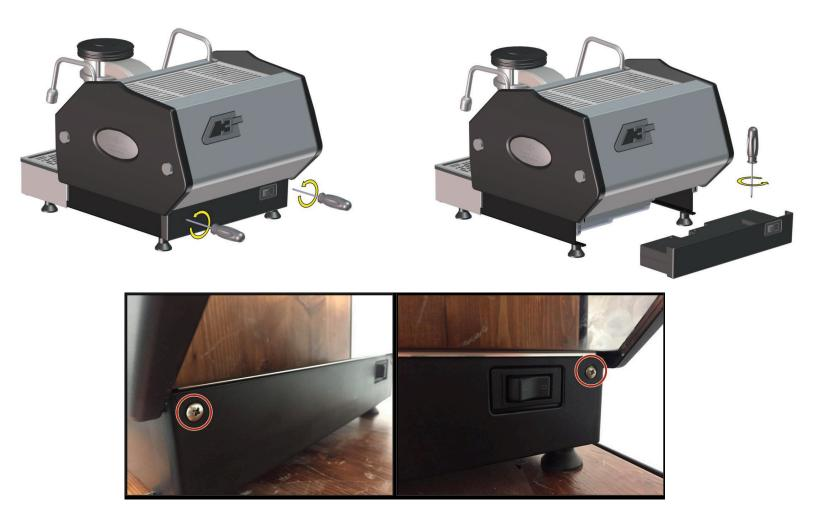
Remove electronic board box. First, remove the screws on the rear of the GS3, then remove the rear panel as well as the left and right panels.
